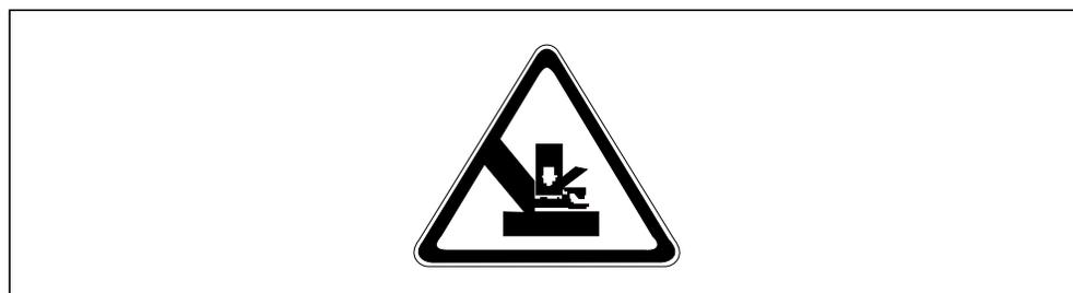
Figure 2-6. The pinching hazard label.
